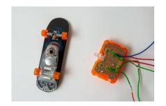
Eyebrow Controlled Skateboard is an arduino hack that allows you to control a miniature RC Skateboard with you're eyebrows. A 'Raise' sends it forward and a 'Frown' sends it backwards using thresholds. Although this example is specific - hacking buttons with arduino is easily replicated with any RC toy...
